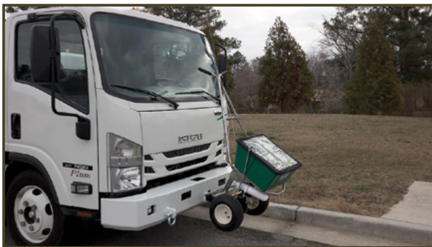
A front-mounted spreader frees up advertising space at the back of the spray rig and lets the driver keep an eye on the cargo.
