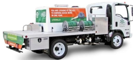
*This dual-system unit features 400-gallon mechanical agitation alongside 200-gallon jet agitation, allowing one rig to service multiple grass types.*
