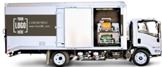
The 18-foot box truck can be outfitted with a variety of Graham spray units. The unit pictured is a 400-gallon tank split 300/100.
